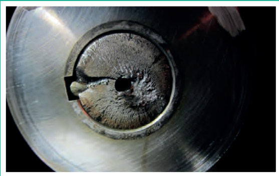
Fatigue crack - turbine side
